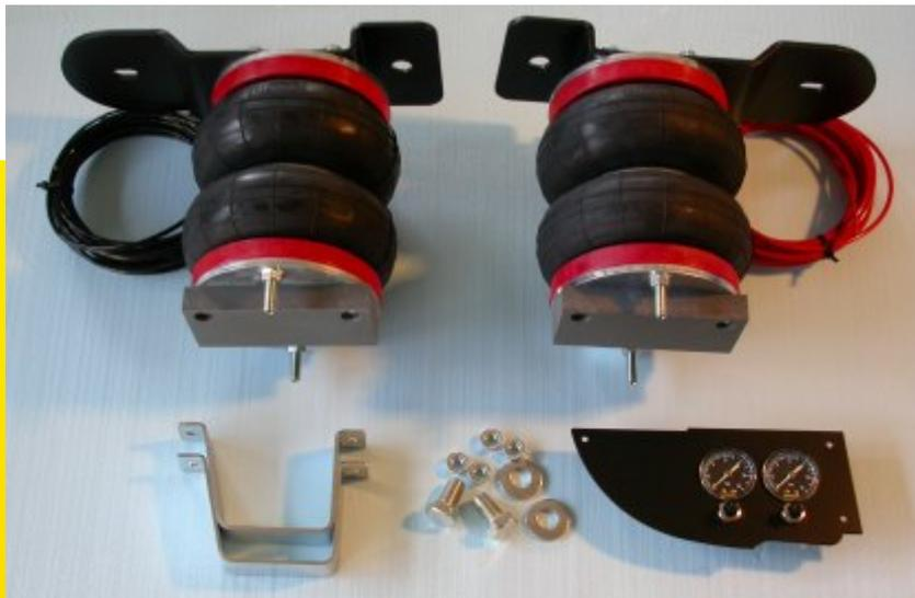
IL COMPLESSIVO "B132" CON IL KIT MANOMETRI "D15" FORNITO DI SERIE
